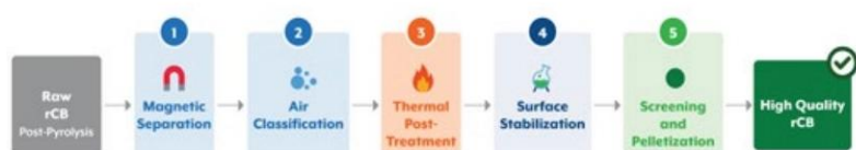
Figure 3. Integrated rCB Upgrading and Purification Process Sequence.
